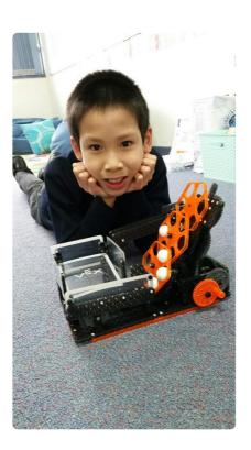
I've been doing robotics at lunchtime this term and I've finally finished what I wanted to build. A Hexalator! It's cool and fun and I enjoyed building it. When you turn the gears the hexagon rotates and carries the balls up and around and then down the track.
